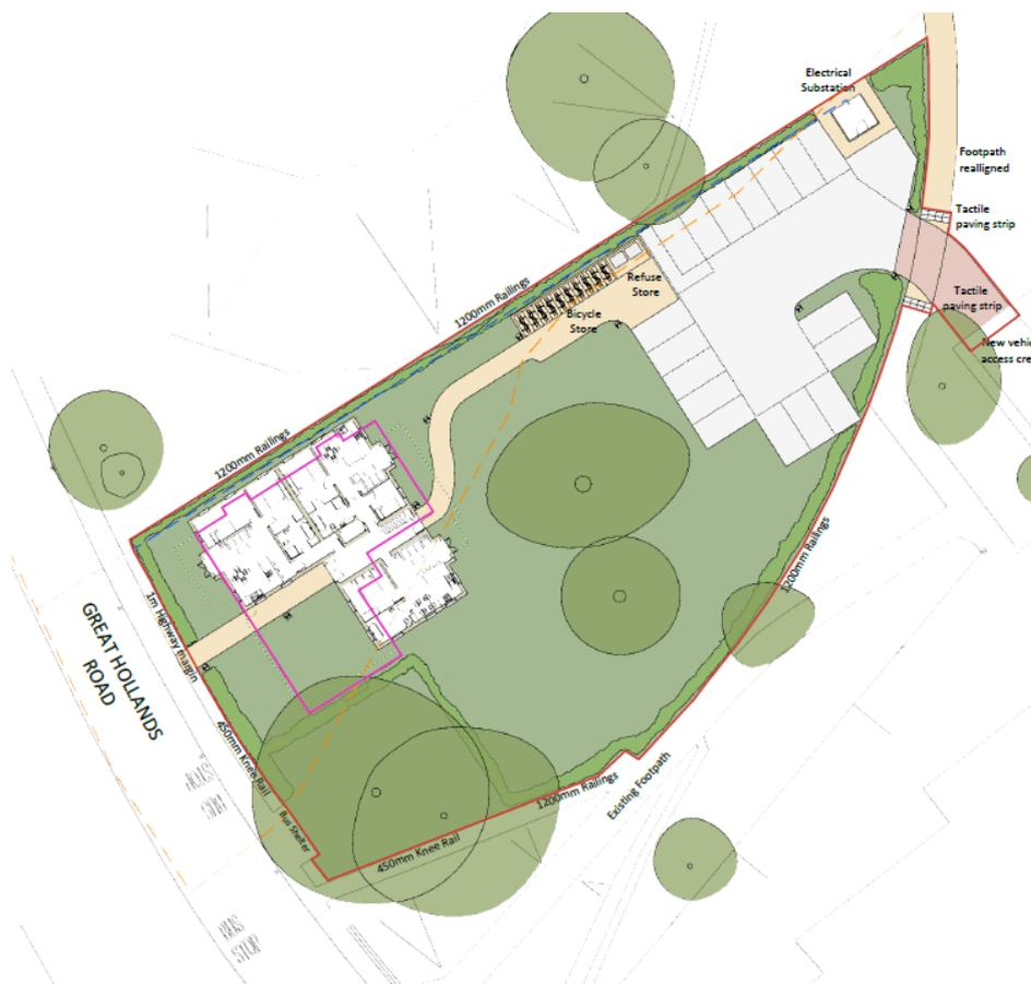
5.3 The building would be 'L-shaped' with a maximum width of 18m and a maximum depth of 16.8m. It would have a height of 10.8m with a hipped roof design and dormers at second floor. The floor plans would follow the same pattern at ground, first and second floor level with 2no. two bedroom flats and 1no. one bedroom flat provided at each level.
